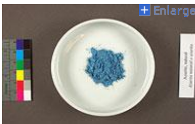
High resolution digital photos are taken of all samples, along with a color test patch. This allows any user to calibrate their monitor in order to accurately view the sample in its "true" colors. Photo: Dusan Stulik.
