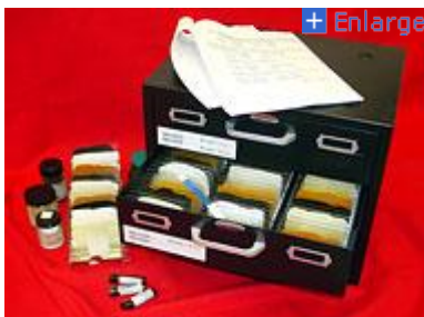
Collection of binary mixtures of binding media, an important tool in developing various analytical methodologies for analysis of artifacts. More than 900 samples were prepared using combinations of different binding media in concentrations ranging from 0.1%–99.9%. Photo: Dusan Stulik.
