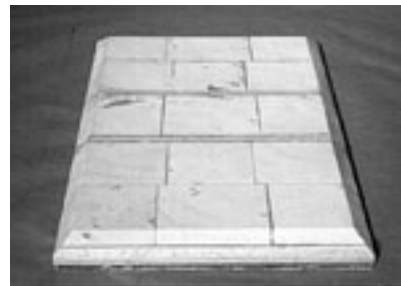
Figure 10 Balsa blocks trimmed and smoothed.
