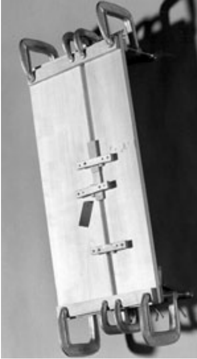
Figure 7 Temporary tiranti, or levers, used to pull distorted surfaces of separated panel boards back into plane before wedges are glued into previously prepared grooves.
