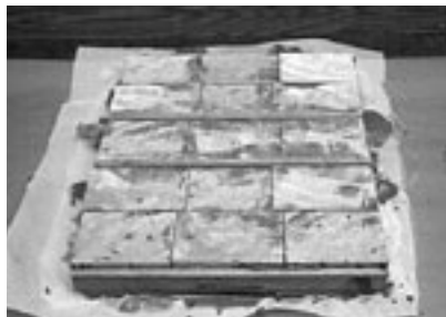
Figure 9 Balsa-block backing in place.
