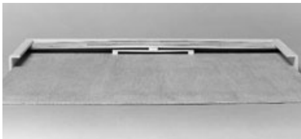
Figure 9, right Model of the spring support assembly with a panel at a neutral curvature profile (55% RH).
