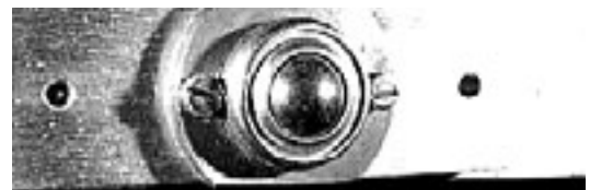
Figure 17 The support bearing seen from below.
