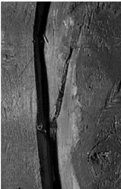
Figure 26 Lorenzo Monaco, The Annunciation . A split on the back of the panel; some ring separation is evident in the wood of the support's central plank.
