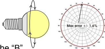
For this type of light source is the "B" field nearly completely circular and therefore is subject to a very small error when measured using the "A" field only.
