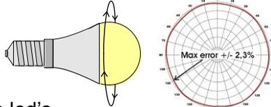
The plastic cone exposes the led's and therefore has a bit more uneven distribution of the "B" field and thus a higher error value.
