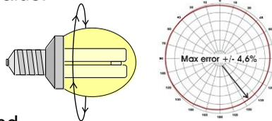
The large field of light from and fluorescent bulb and the uneven wear of the glass tubes increases the error of measurement compared to LED.
