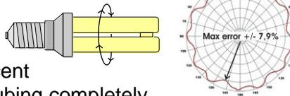
Non-frosted coned fluorescent bulb exposures the glass tubing completely and therefore produces an oscillating "B" field depending on the number of tubes.
