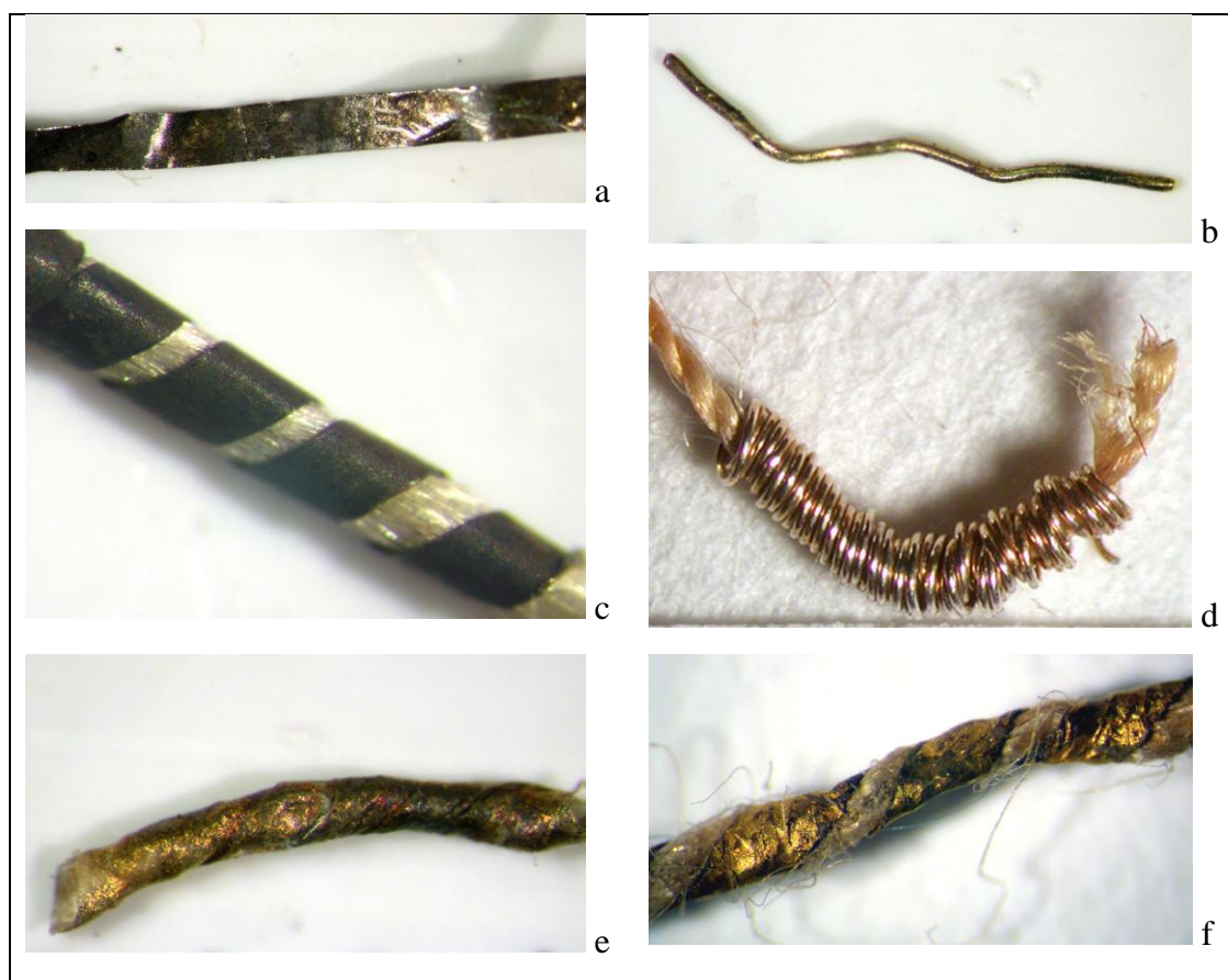
Fig. 1: Types of metal threads: a) metal strip, b) wire, c) strip wound around a silk yarn, filé ; d) spiral wire, tir-tir ; e) gilt membrane strip spun around a silk yarn, and f) gilt leather strip wound around a silk yarn. OM images, (mag. x40).
